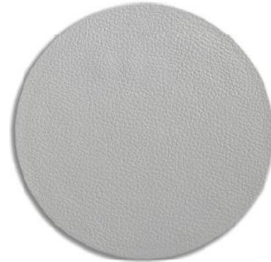
HYDRO PU coating after cleaning
