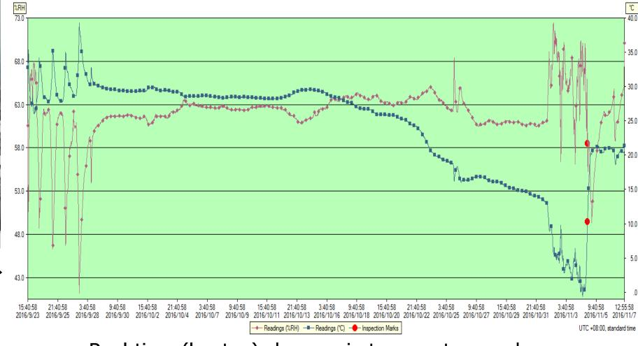
Real-time (log tag) changes in temperature and humidity inside the container during a 46-day ocean transit.
